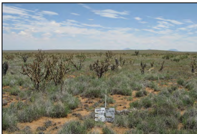
Figure 13. Example photo point picture. Transect tape is straight and threaded below vegetation, Photo ID board is in the bottom center of the photograph, and the horizon is in the background.
