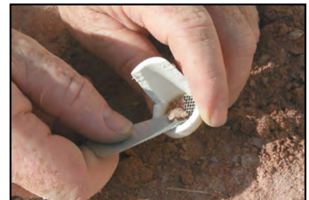
Figure 26. Place sample in sieve.
