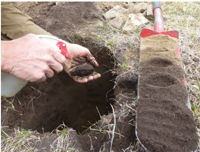
Figure 11. Removing samples by horizon from the soil pit allows the observer to easily describe the color, texture, effervescence, and percent clay content for each horizon.
